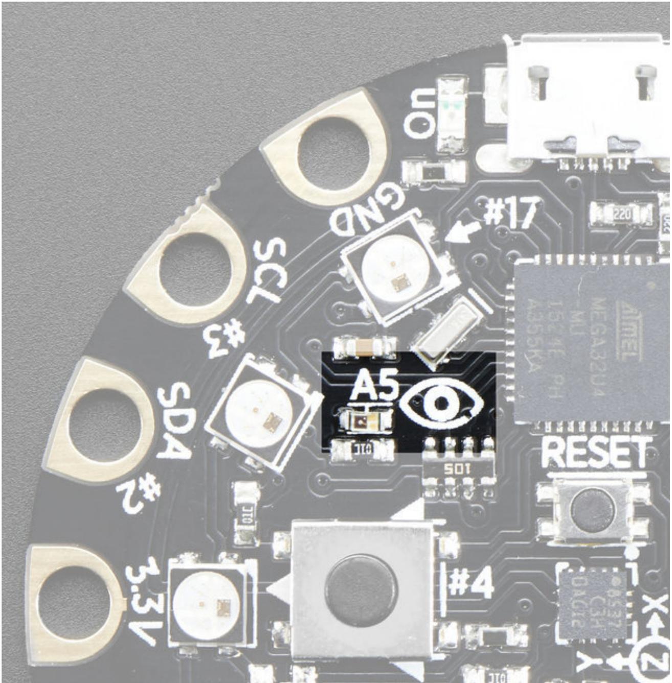
There is an analog light sensor, [part number ALS-PT19](#), in the top left part of the board. This can be used to detect ambient light, with similar spectral response to the human eye.
