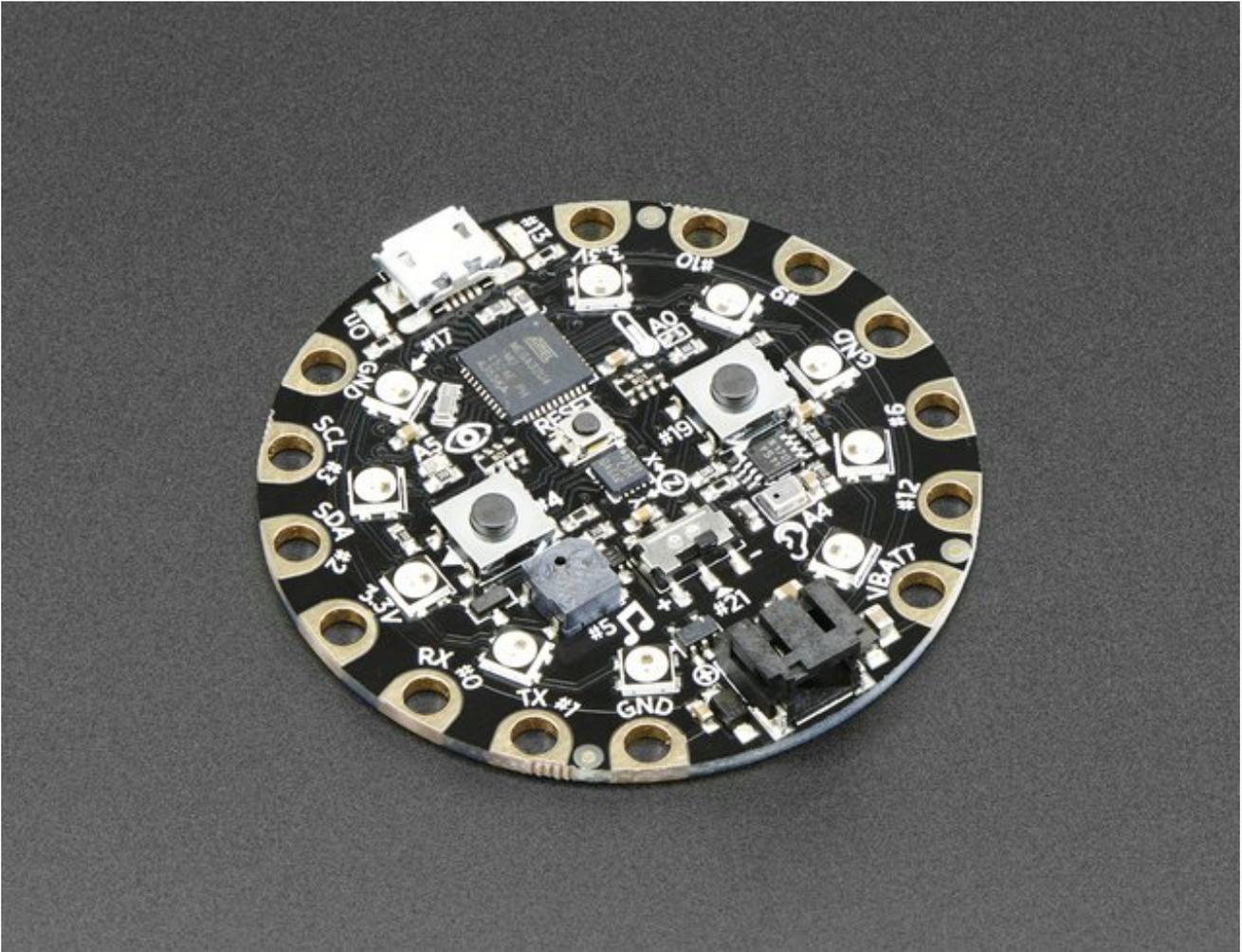
Circuit Playground has built-in USB support. Built in USB means you plug it in to program it, it just shows up - all you need is a Micro-B USB cable, no additional purchases are needed! [With the new 1.6.4+ Arduino IDE, it takes only a few seconds to add support \(http://adafru.it/nb4\)](http://adafru.it/nb4). The Circuit Playground has USB HID support, so it can act like a mouse or keyboard to attach directly to computers.
