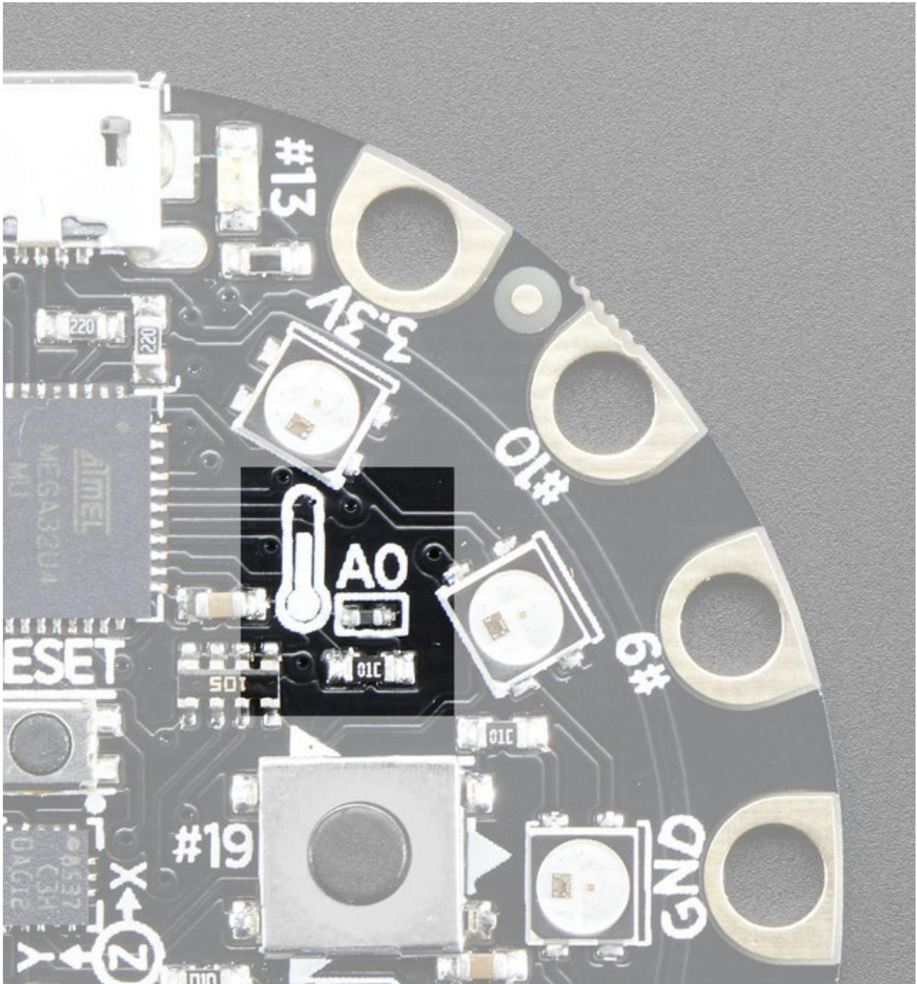
There is an NTC thermistor ([Murata NCP15XH103F03RC](https://www.murata.com/en-us/products/ntc-thermistors/ntc-thermistors-series/nct15xh103f03rc)) that we use for temperature sensing. While it isn't an all-in-one temperature sensor, with linear output, it's easy to calculate the temperature based on the analog voltage on analog pin **#A0**. There's a 10K resistor connected to it as a pull down.
